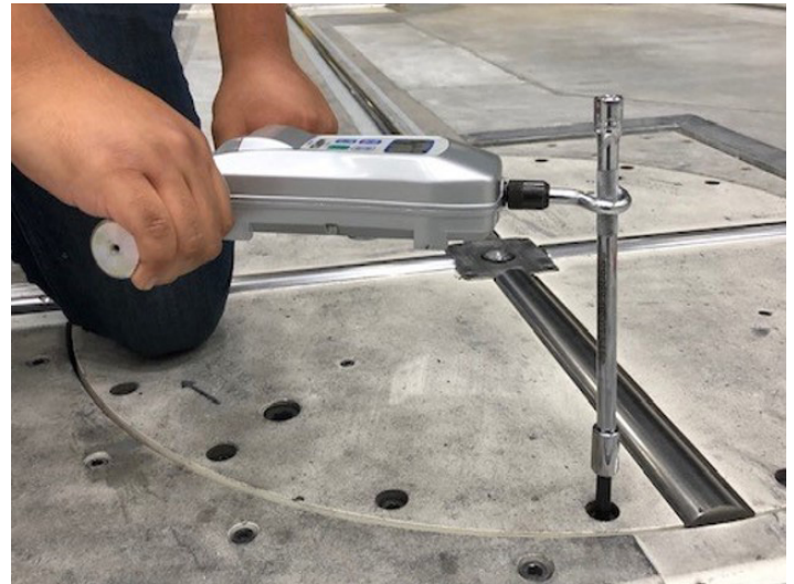
Figure 2: Technician Measuring the Operational Torque of a Turntable
